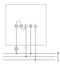
The device can be manually activated with a circuit breaker. After releasing the button (return of power) the device switches on (for at least 40 secs or for the time set on the device).
