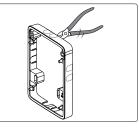
If applicable, use optional corner bracket (9070904, 9070905) or spacer frame (9070908, 9070909) for flexible installation as well as cable entry from side or top/bottom.
